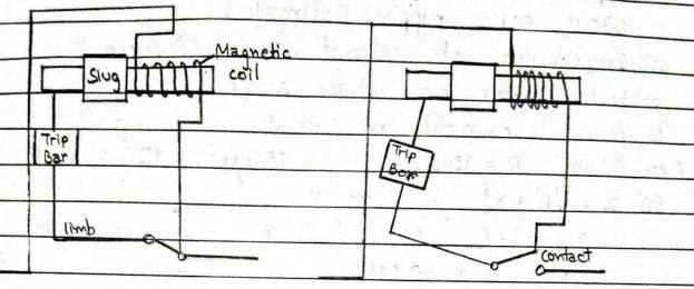
In some MCBs, magnetic field generated by coil causes / develops pull on trip bar so that the contact get open.
